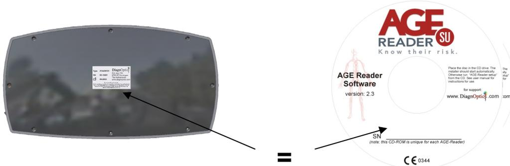
**2.** To install you need to have administrator rights. Insert the AGE-Reader CD in the CD/DVD-drive of a computer running 32-bit Windows 2000 or later. The installer should start automatically, otherwise run "setup23-eng.exe" from CD.
